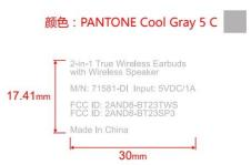
Note: The Earbuds do not contain enough place for the label. The label is place on the speaker(charging for the earphone) together used with the earpone
