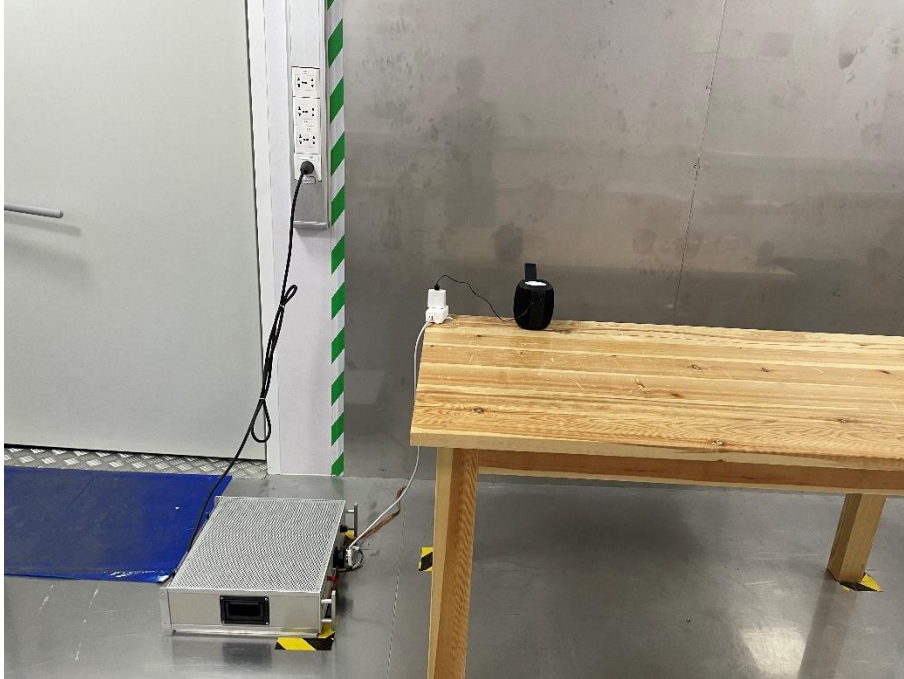
Band edge emissions (Radiated) Emissions in restricted frequency bands (above 1GHz)
