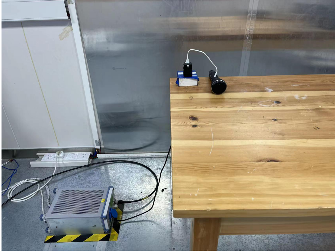
Conducted emission test setup
