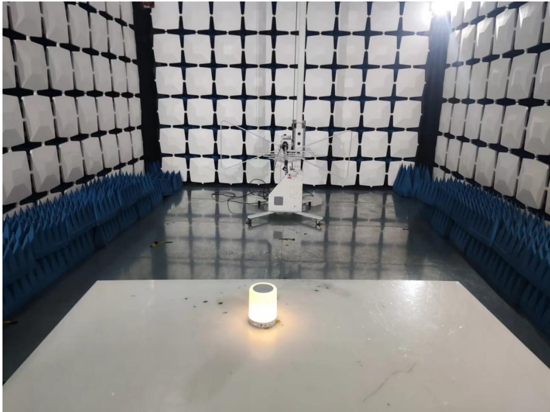
Blow 1GHz for radiated emission test setup
