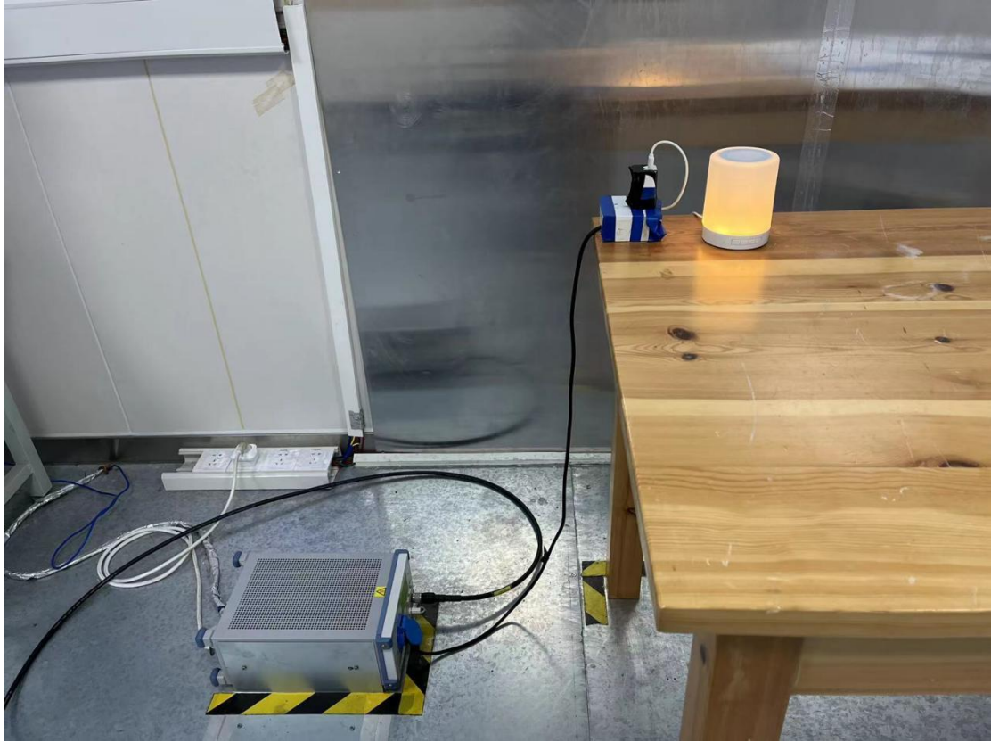
Conducted emission test setup
