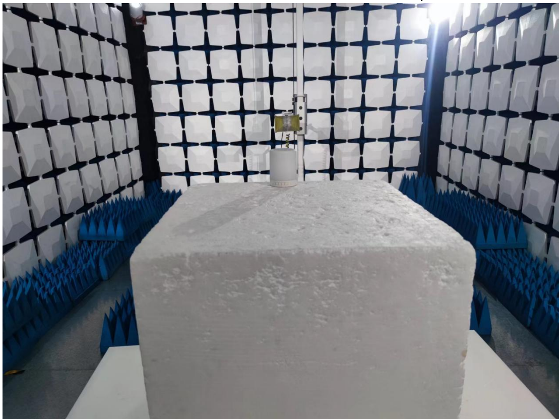
Above 1GHz for radiated emission test setup
