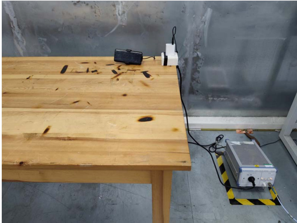
Photo of Conducted Emissions Measurement
