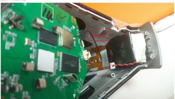
The antenna is integrated on the main PCB and no consideration of replacement. The best case gain of the antenna is 1.56dBi.
