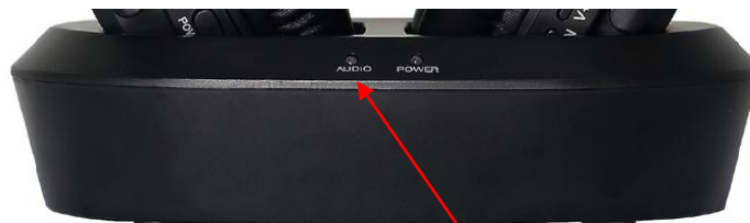
AUDIO LED turn blue if signal come through
