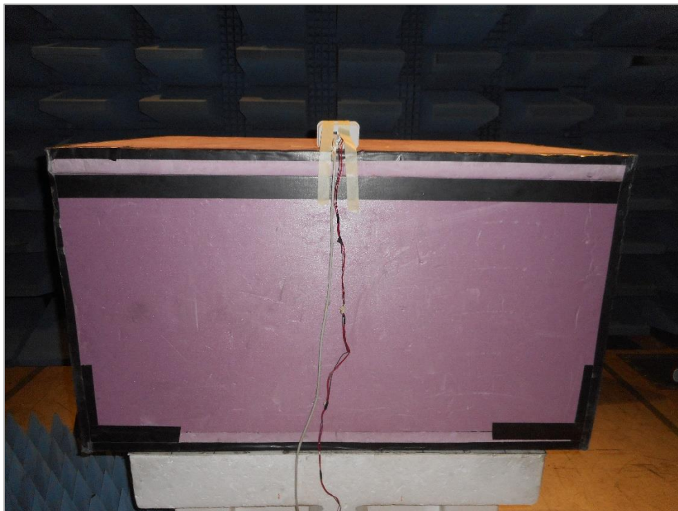
Figure 4: Radiated Emissions performed above 1GHz (close-up view) Test Setup
