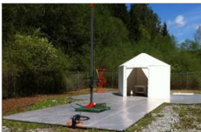
10m Open Area Test Site (OATS) in British Columbia, Canada
