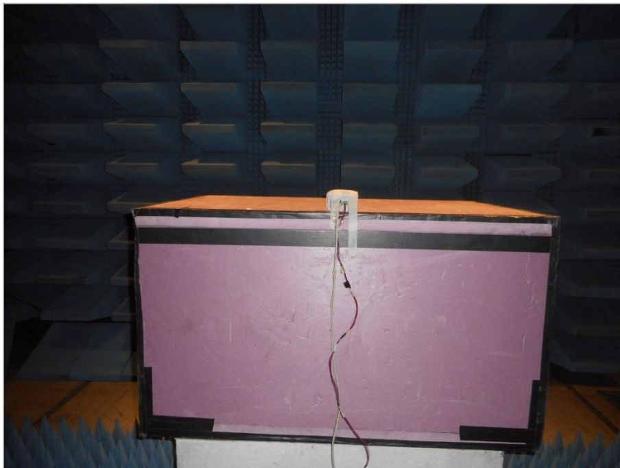
Figure 4: Radiated Emissions (above 1 GHz, close-up view) performed at the SAC Test Setup
