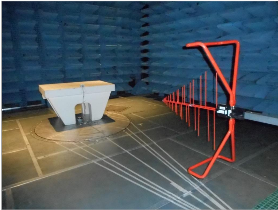
Figure 1: Radiated Emissions (below 1 GHz) performed at the SAC Test Setup
