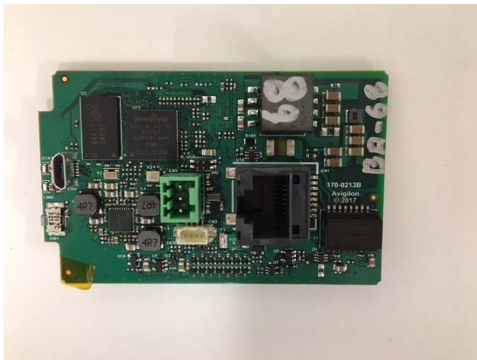
Avigilon Processor Board Top View:
