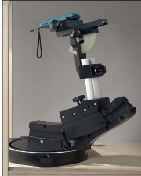
F-2. Device Holder for Transmitters
