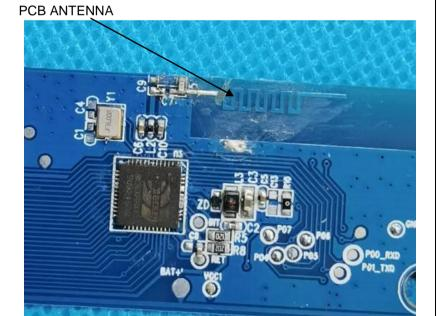
The antenna is integral antenna. The best case gain of the antenna is 0dBi.
