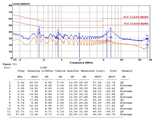
Remarks: 1. Measured = Reading + LISNFac + Cable Loss + Aux2 Fac. 2. The emission levels that are 20dB below the official limit are not reported.
