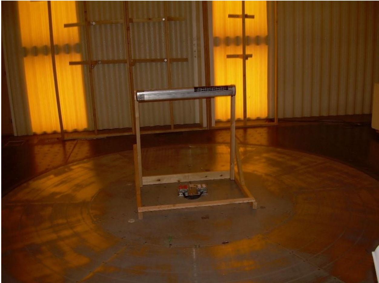
Photograph 1. Front View Radiated Emissions 30 to 1000 MHz Range – Awning Retracted
