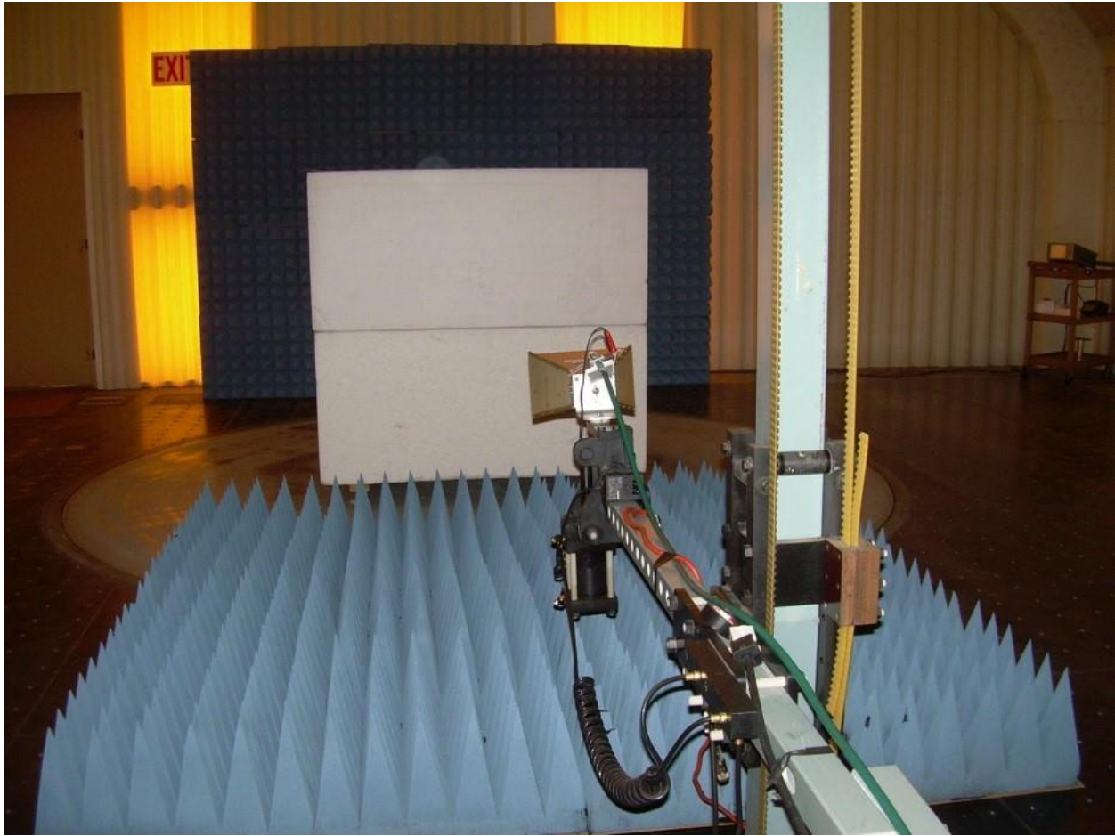
Photograph 7. Test Setup for Emissions Above 1000 MHz
