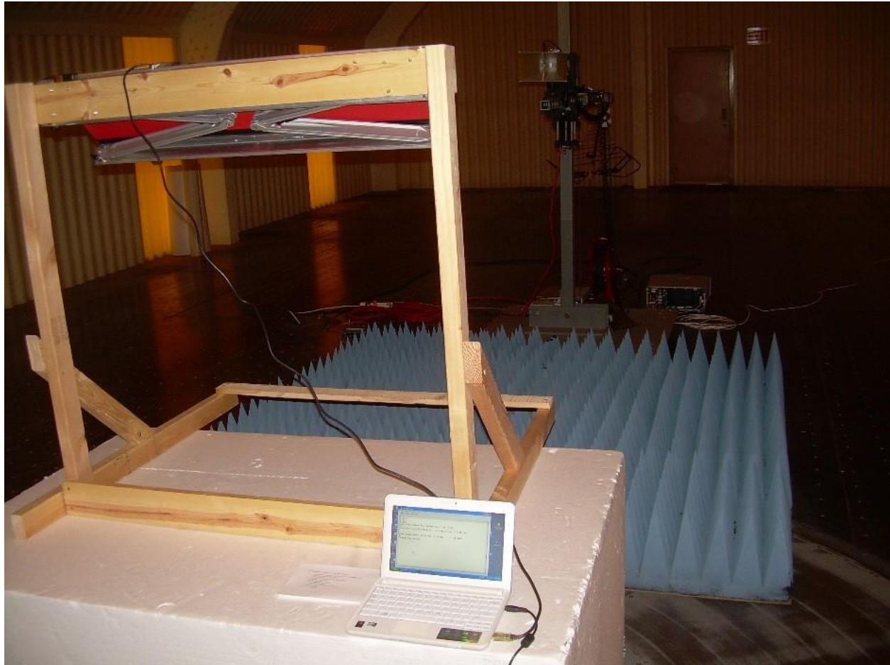
Photograph 4. Back View Radiated Emissions Above 1000 – 12400 MHz Range – Awning Extended
