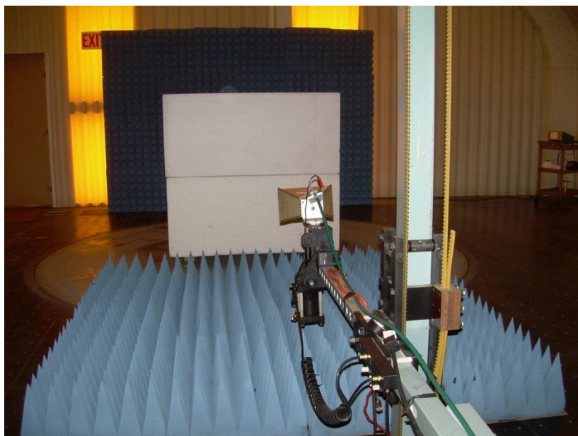
Photograph 19: Test Setup for Emissions Above 1000 MHz
