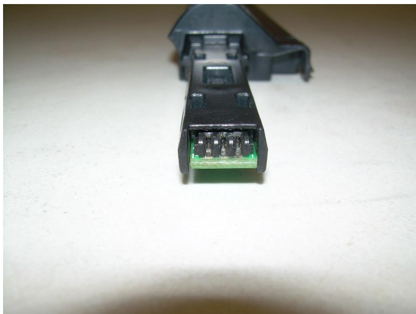
Photograph 12 – View of the Battery Connector
