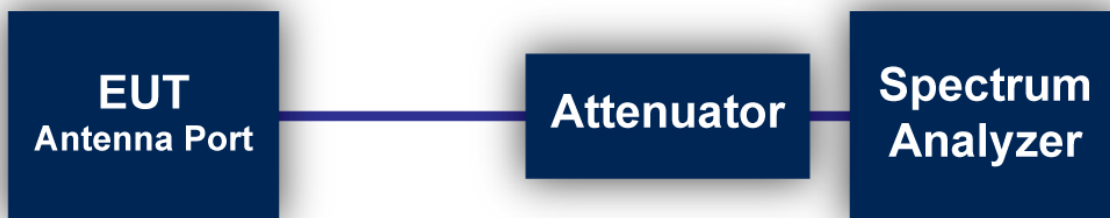
Figure 1: Direct Connection at the Antenna Port Test
