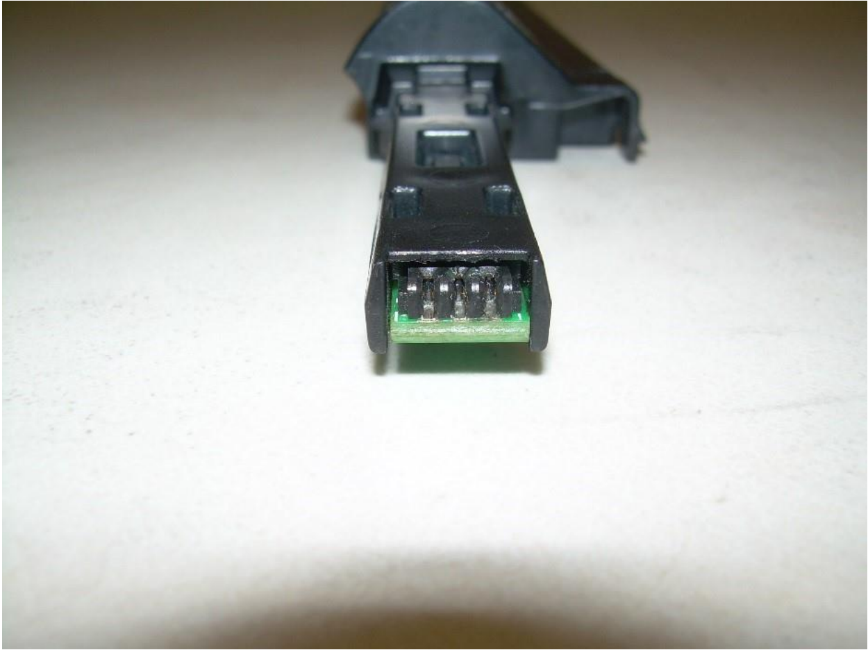
Photograph 5 – View of the Battery Connector
