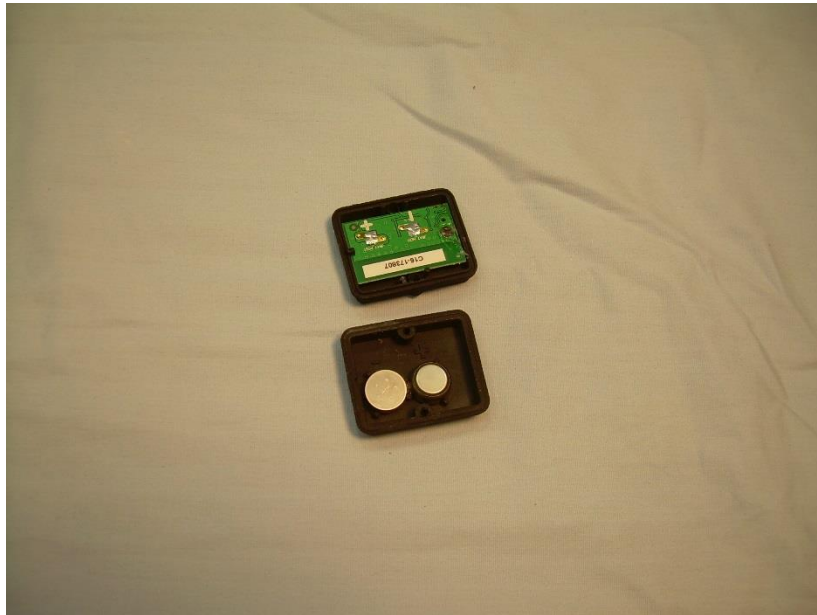
Photograph 10 – View of the Housing Open Showing PCB and Battery Placement
