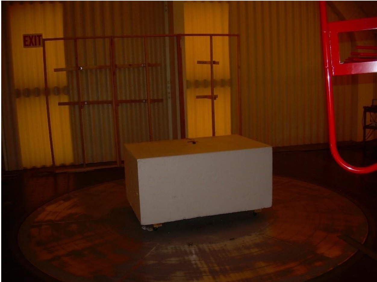
Photograph 1. Front View Radiated Emissions – Below 1000 MHz Configuration
