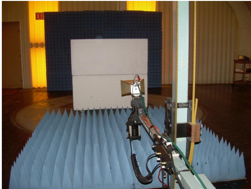
Photograph 16: Test Setup for Emissions Above 1000 MHz
