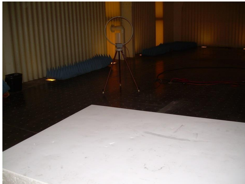
Photograph 14: Test Setup for Emissions Below 30 MHz
