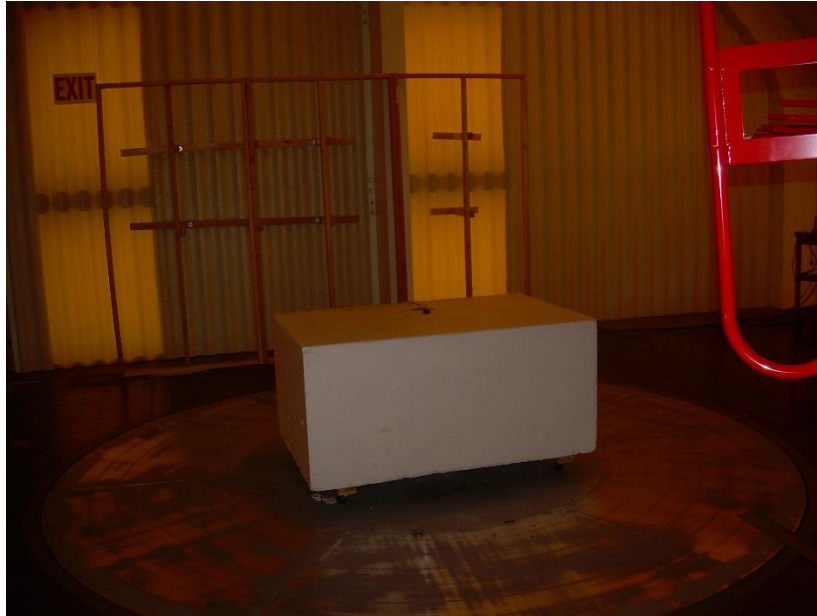
Photograph 1: Front View Radiated Emissions – Below 1000 MHz Configuration
