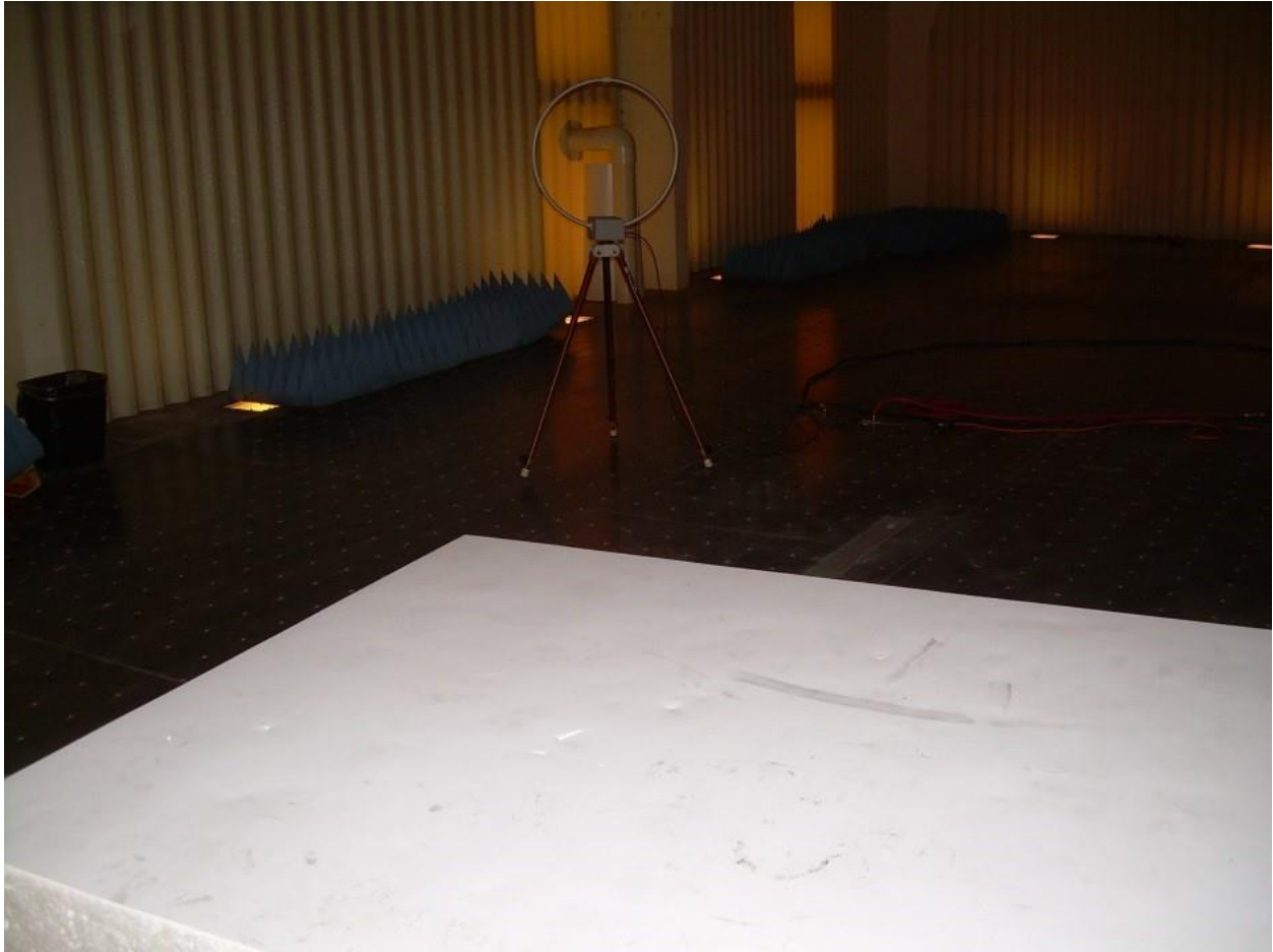
Photograph 10. Test Setup for Emissions Below 30 MHz
