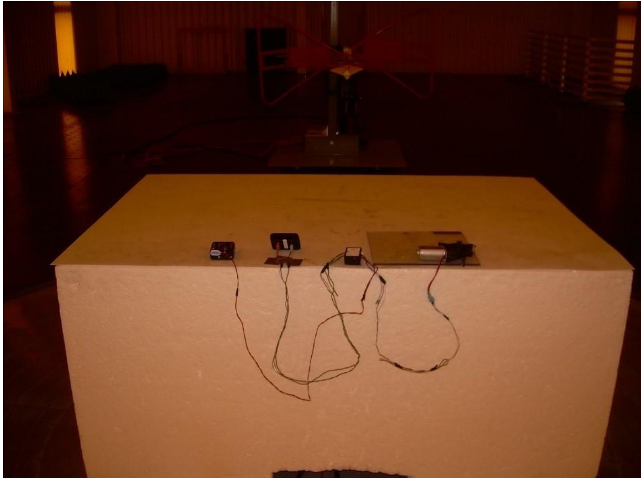
Photograph 4. Back View Radiated Emissions 30 to 1000 MHz Range
