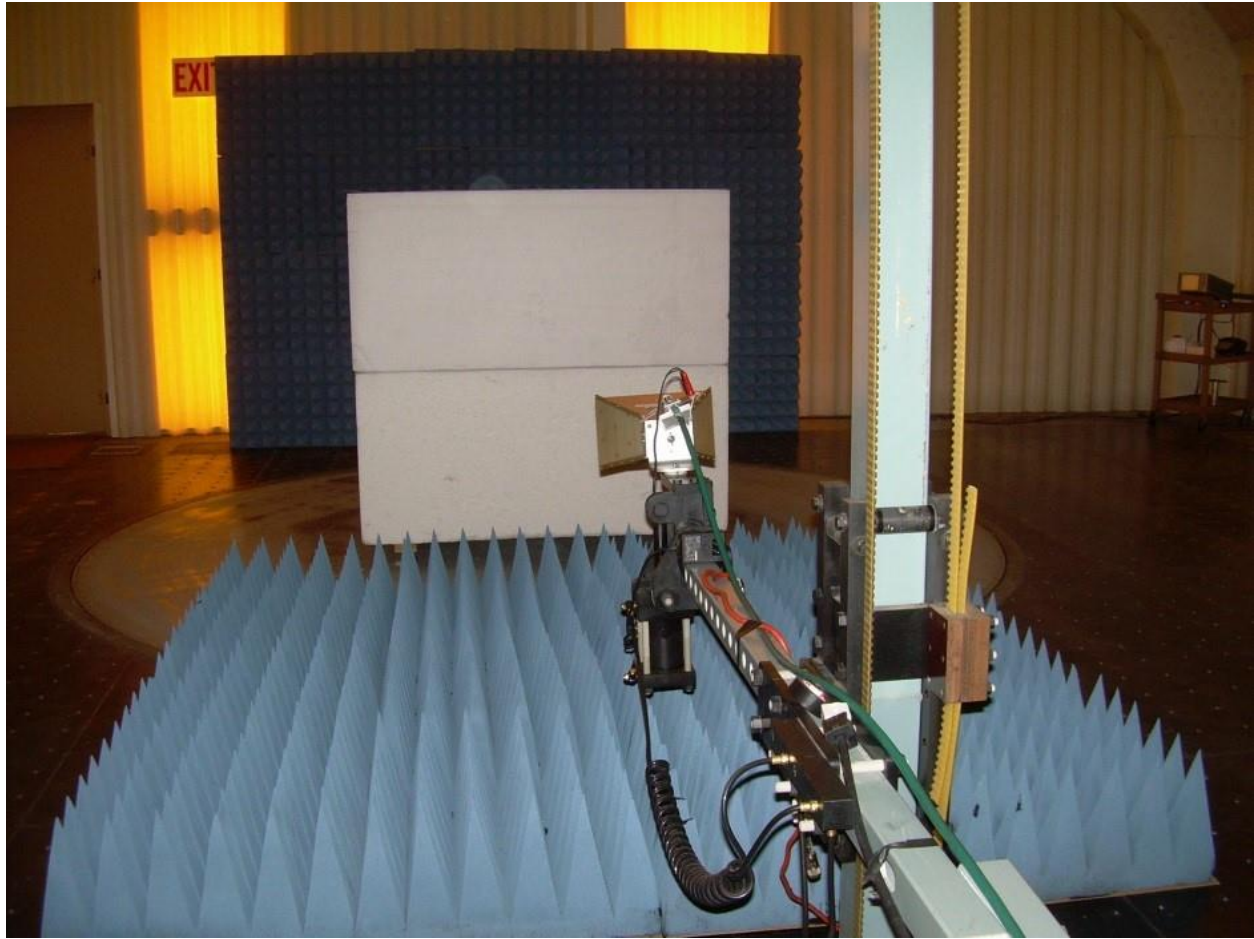
Photograph 12. Test Setup for Emissions Above 1000 MHz
