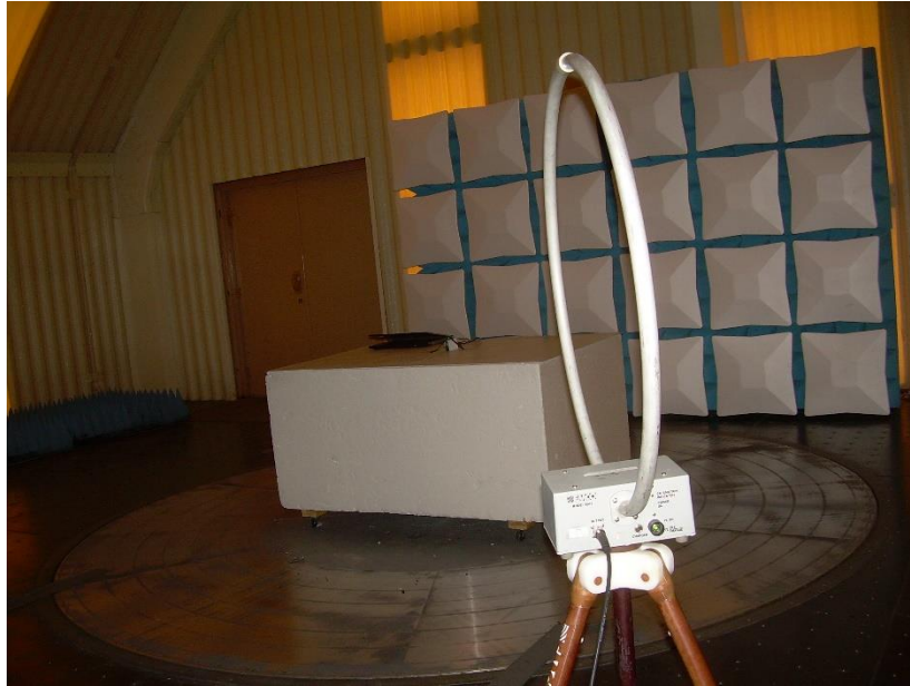
Photograph 1: Front View Radiated Emissions Configuration – Below 30 MHz
