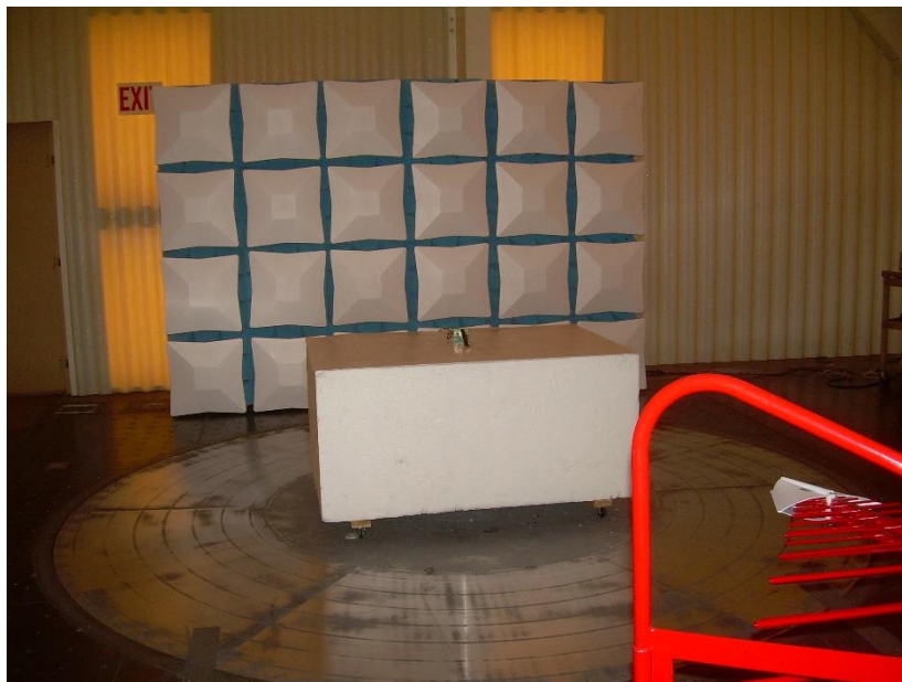
Photograph 2: Front View Radiated Emissions Configuration - 30 MHz – 1000 MHz
