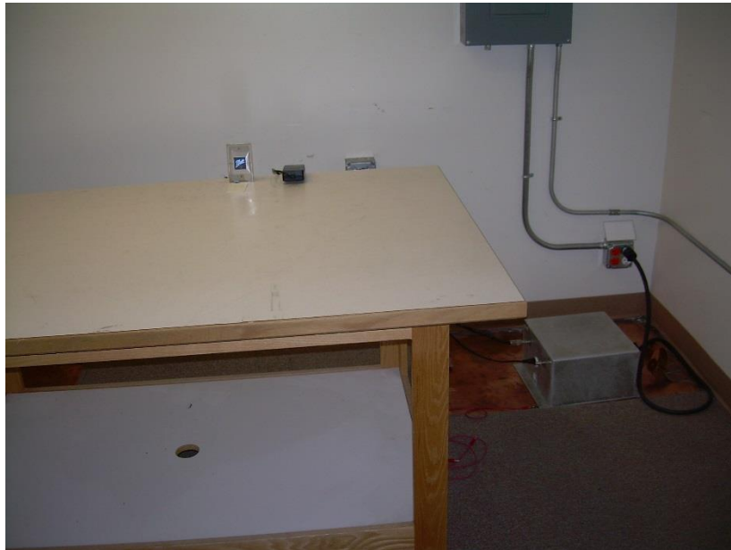
Photograph 6 – Front View Conducted Emissions Worst-Case Configuration
