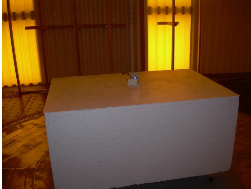
Photograph 1 – Front View Radiated Emissions Worst-Case Configuration – Vertical Placement
