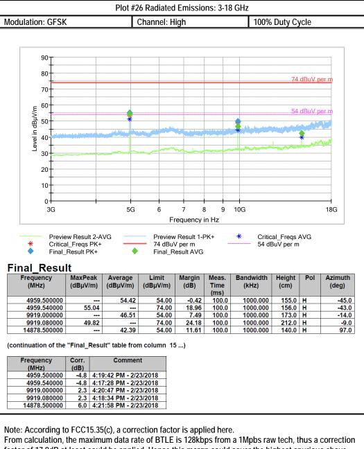
factor of 17.9dB at least could be applied. Hence this margn could cover the highest spurious above.
