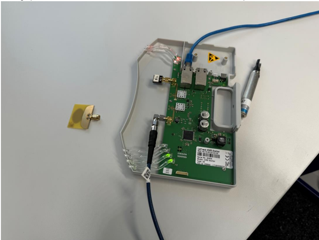
Photograph 11: conducted measurement with RF cable connected at UWB port. Close view.
