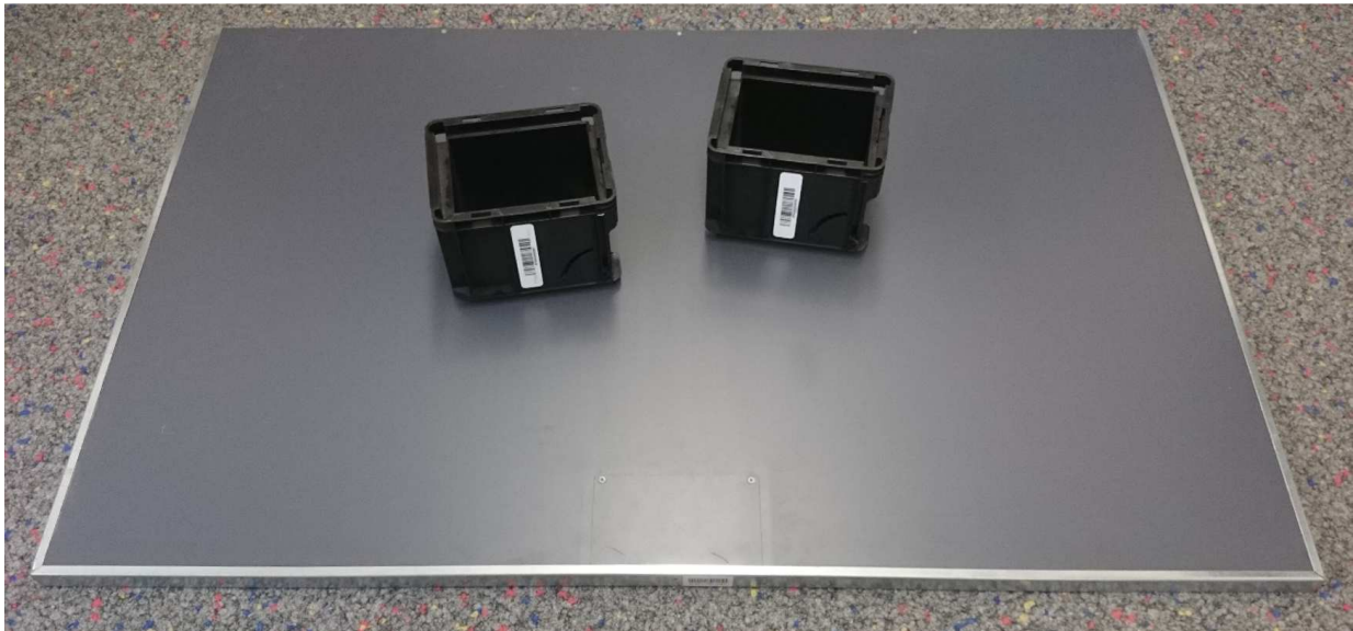
Figure 4: LeanOrder detectionShelf with two RFID-labeled empty bins
