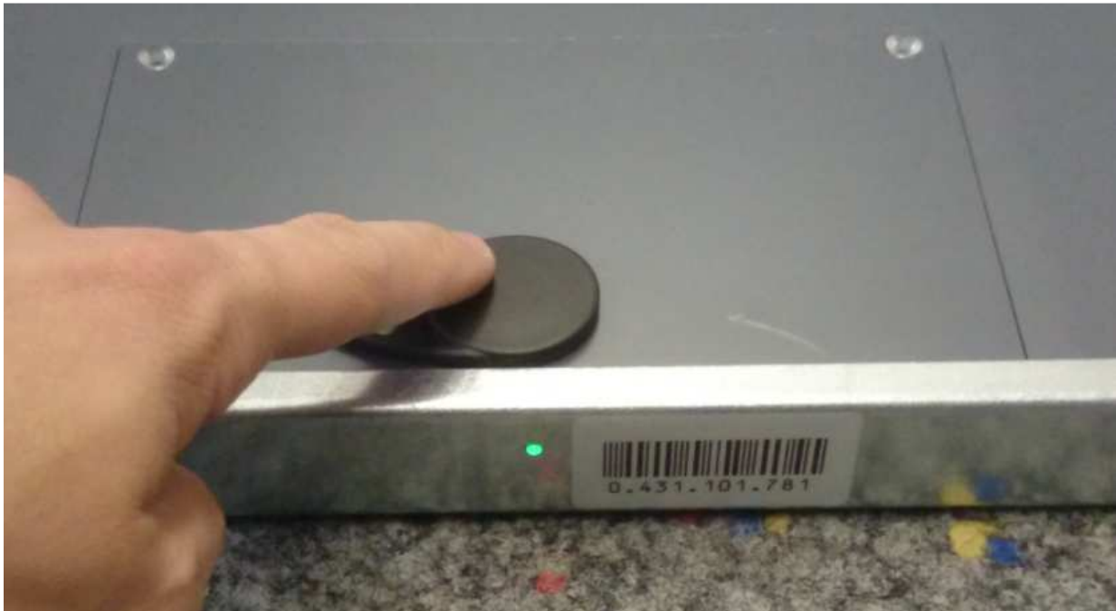
Figure 5: A magnet on the LeanOrder detectionShelf to trigger the manual scanning mode
