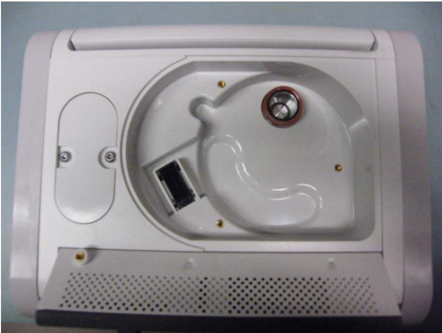
Figure 10: Rear View of OBM version Trilogy EVO with OBM module removed
