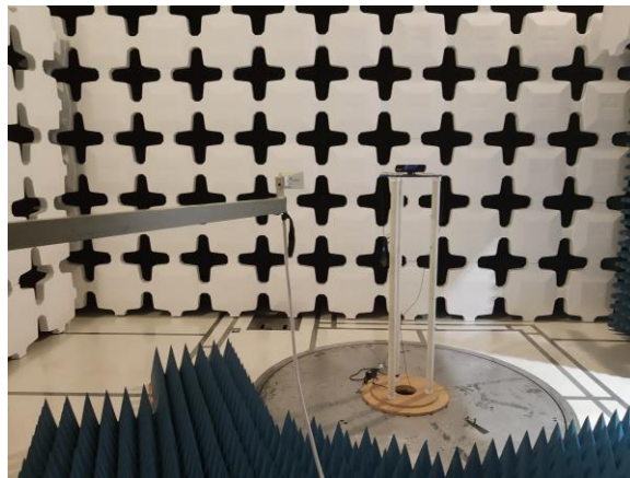
Figure 43: REE Test Setup - 18-25 GHz
