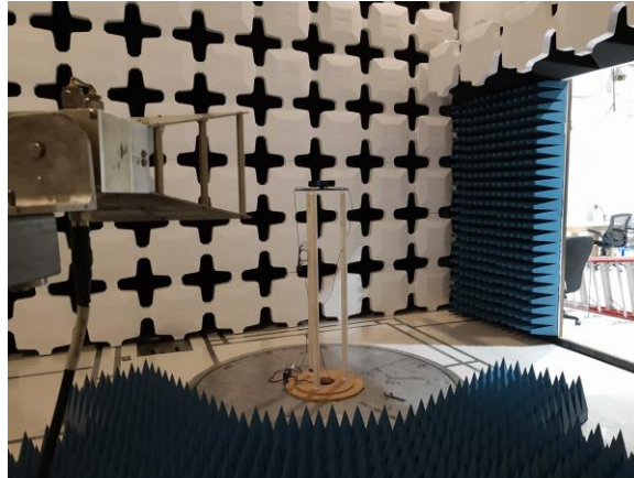
Figure 42: REE Test Setup - 1-18 GHz
