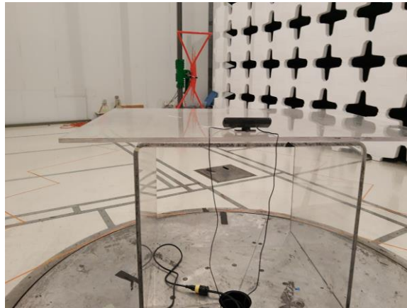
Figure 41: REE Test Setup - 30-1000MHz
