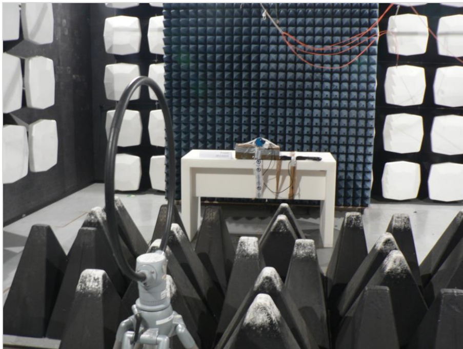
Photograph 4: EUT test setup in the semi-anechoic chamber. Tested frequency range below 30 MHz
