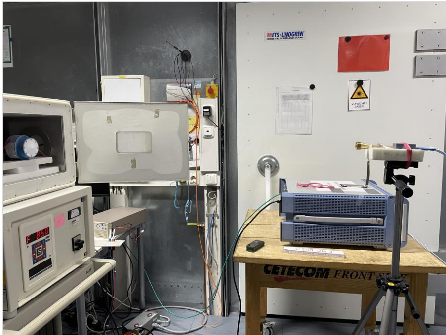
Photograph 3: EUT test setup in the climatic chamber for test under extreme conditions
