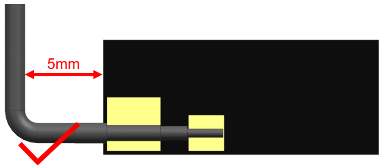
FIGURE 5.2.1 RECOMMENDED CABLE BENDING RANGE
