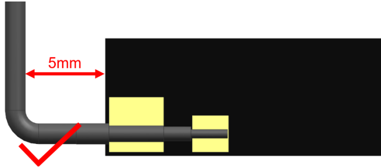
FIGURE 5.2.1 RECOMMENDED CABLE BENDING RANGE
