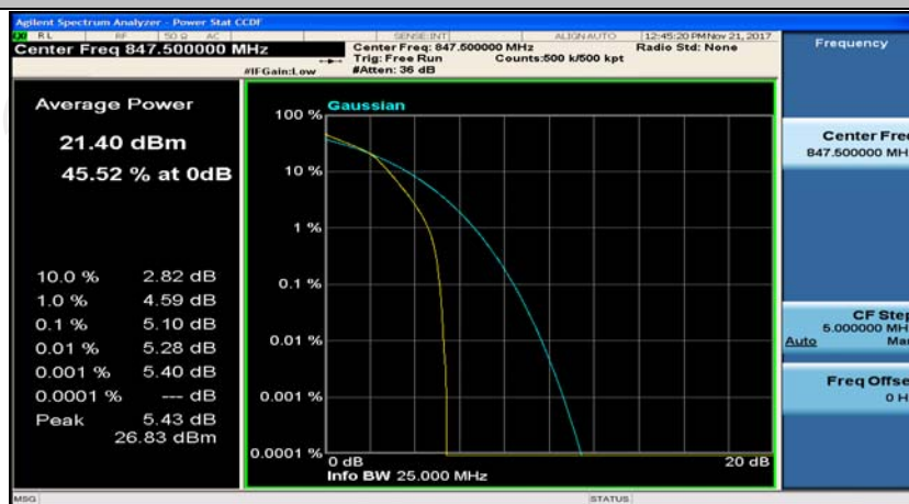
(Channel Bandwidth: 3 MHz)_HCH_16QAM_8RB#4
