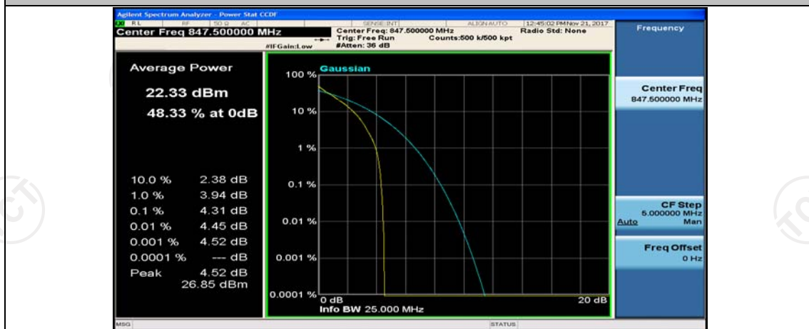
(Channel Bandwidth: 3 MHz)_HCH_QPSK_8RB#4
