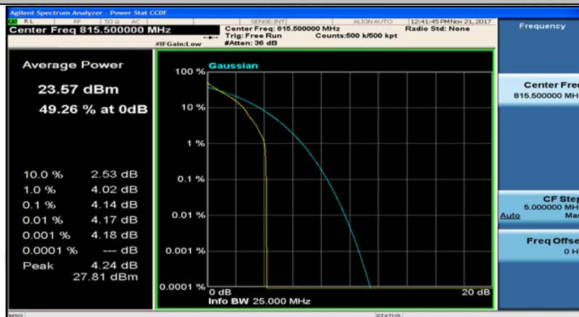
(Channel Bandwidth: 3 MHz)_LCH_QPSK_8RB#0
