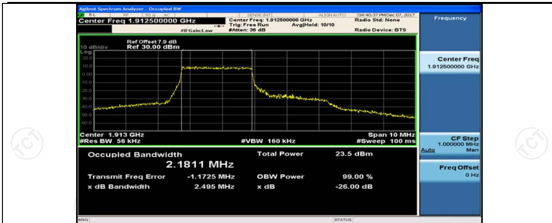
(Channel Bandwidth: 5 MHz)_HCH_16QAM_12RB#6
