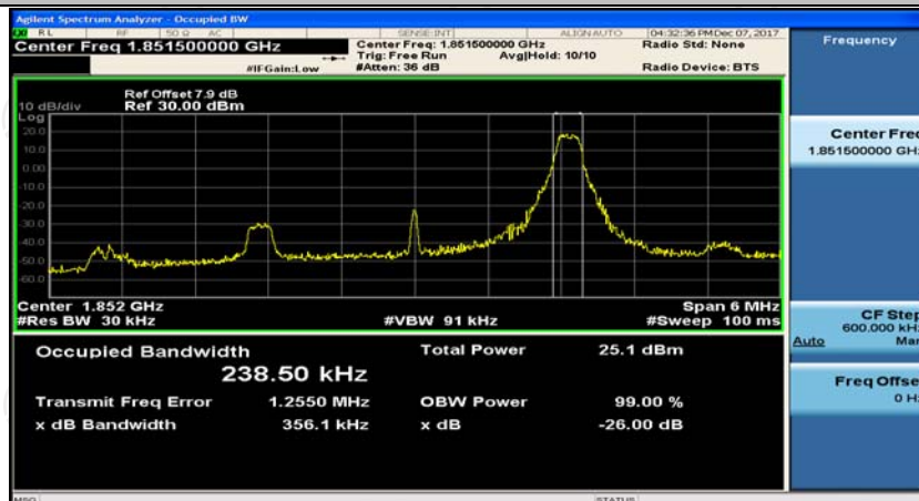
(Channel Bandwidth: 3 MHz)_LCH_16QAM_1RB#14
