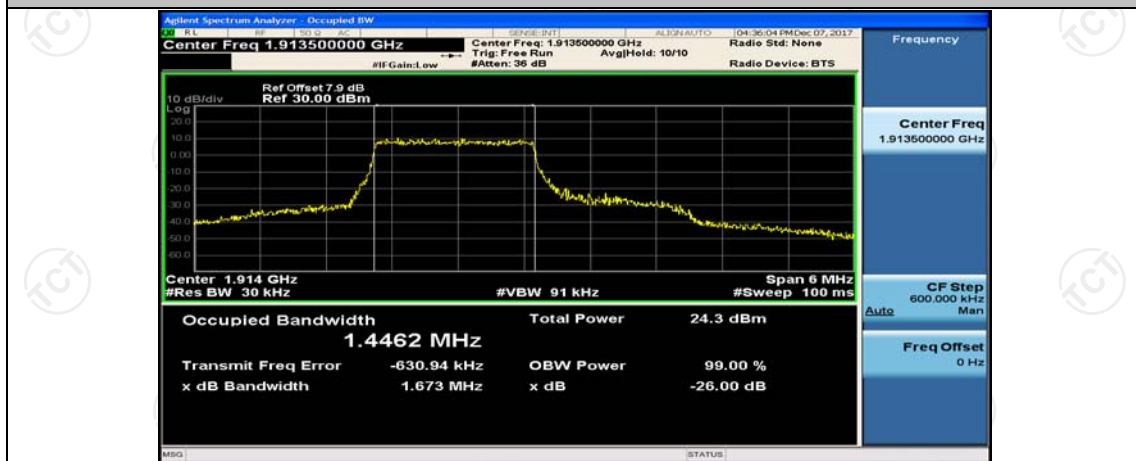
(Channel Bandwidth: 3 MHz)_HCH_16QAM_8RB#4
