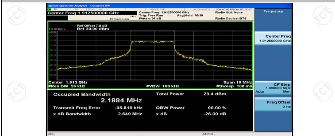
(Channel Bandwidth: 5 MHz)_HCH_16QAM_12RB#13
