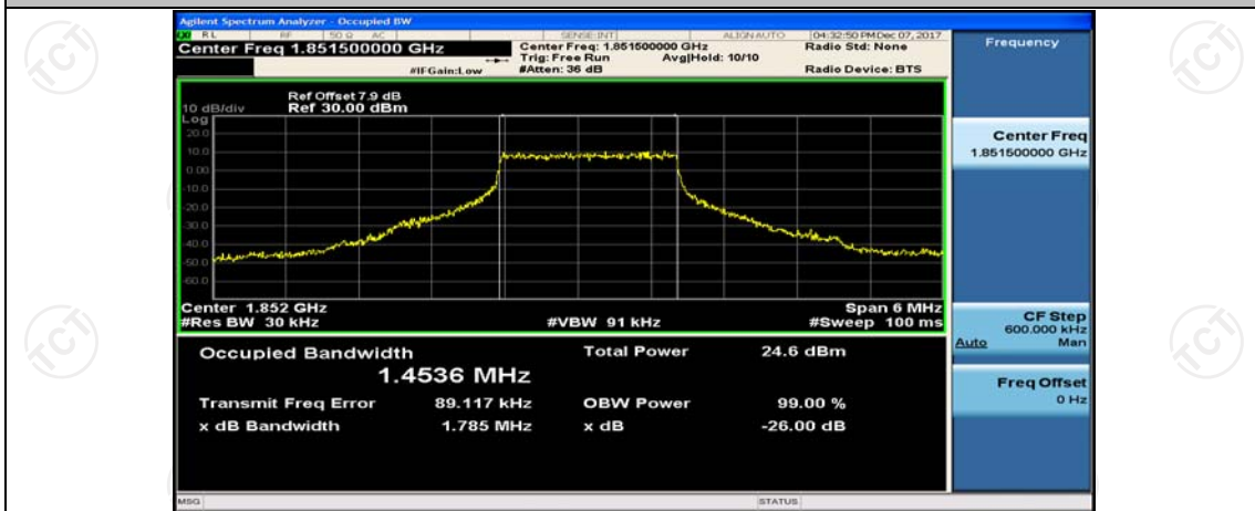
(Channel Bandwidth: 3 MHz)_LCH_QPSK_8RB#7
