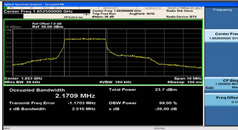
(Channel Bandwidth: 5 MHz)_LCH_QPSK_12RB#6
