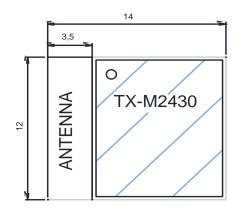
11. 2 Module position on Target board
