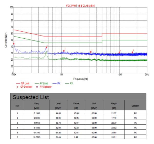
Remark: Transd = Cableloss + Antenna factor - Pre-amplifier; Margin = Limit - Level
