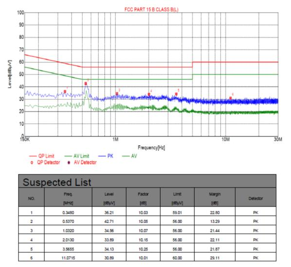
Remark: Transd = Cableloss + Antenna factor - Pre-amplifier; Margin = Limit – Level
