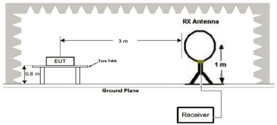
(2) Radiated Emission Test-Up Frequency 30MHz~1GHz
