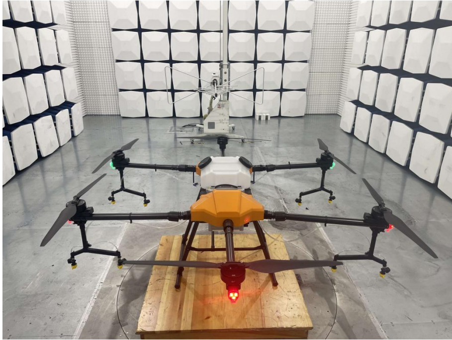
RADIATED EMISSION MEASUREMENT (below 1G)
