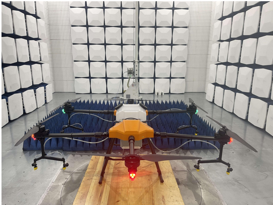
RADIATED EMISSION MEASUREMENT (Above 1G)
