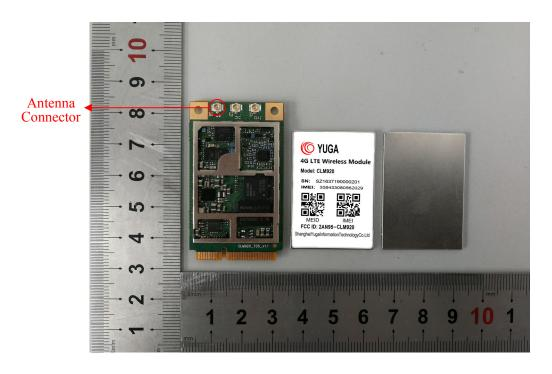
**EUT – Top Shielding off View**
