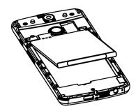
4. Lastly, replace the back cover by aligning the tabs on the cover into the slots on the phone. Gently press the cover until it snaps in place.
