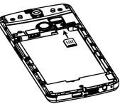
3. Insert the battery by placing the upper section first, with the connection pads at the top left, then click the battery into place.
