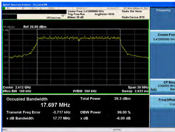
(802.11n20) 6dB Bandwidth plot on channel 1
