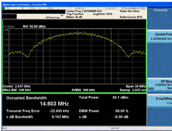
(802.11b) 6dB Bandwidth plot on channel 11
