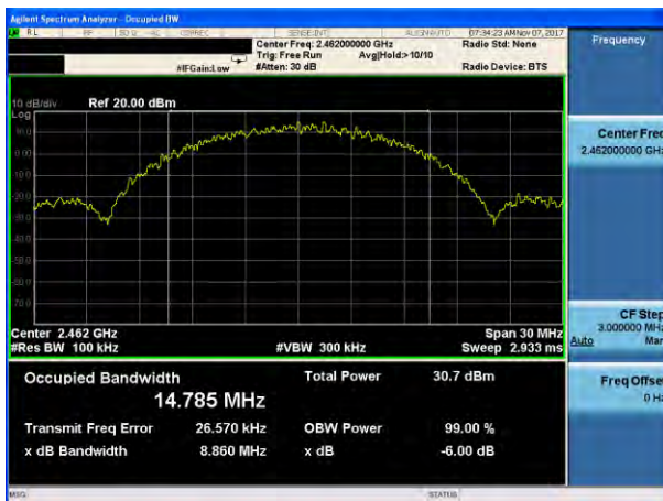
(802.11b) 6dB Bandwidth plot on channel 11
