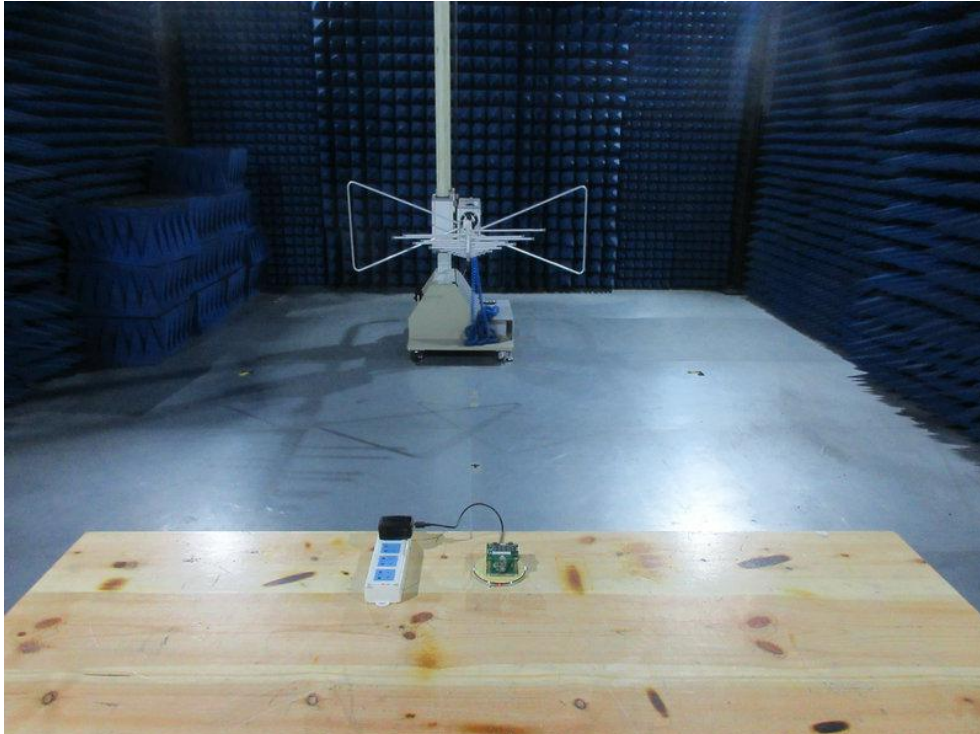
Photo of Radiation Emission Test
