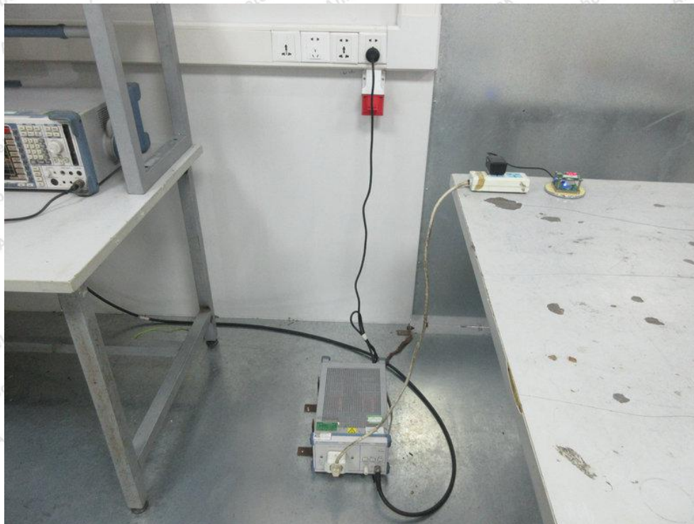
Photo of Conducted Emission Measurement
