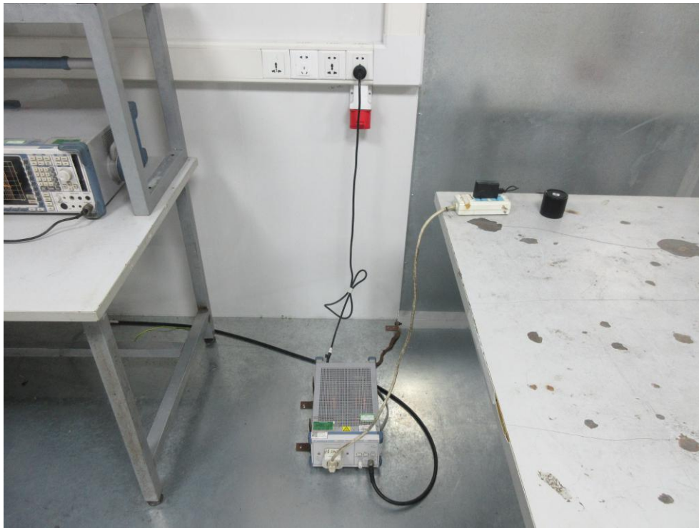
Photo of Conducted Emission Measurement
