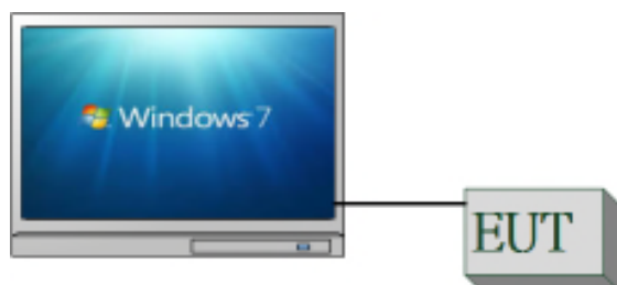
Fig. 2-1 Conducted (Antenna Port) Emission Configuration
