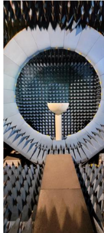
Figure 5-4 Satimo SG-23 6 GHz Stargate Antenna Test Chamber.
