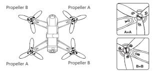
If propellers need to be changed out, please remove the propeller screws first before taking the existing propeller off.
