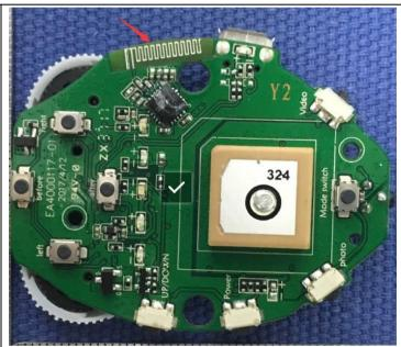
The antenna is integrated on the main PCB and no consideration of replacement. The best case gain of the antenna is 1.0dBi.
