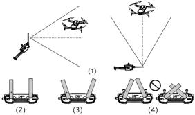
(1) Adjust the angle of the remote control antenna and let it face the flight direction of the aircraft as much as possible.
