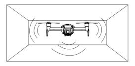
Forward and Backward Vision Systems manually switched on in normal or film mode (Choose to avoid obstacles or actively brake on X-HUBSAN 2.0 APP). Using the Forward and Backward Vision Systems,the aircraft can actively brake when detecting obstacles in front.The Forward and Backward Vision Systems work best with adequate lighting and clearly marked or textured obstacles.
