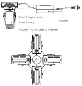
Figure2 - Three battery version( charging)
