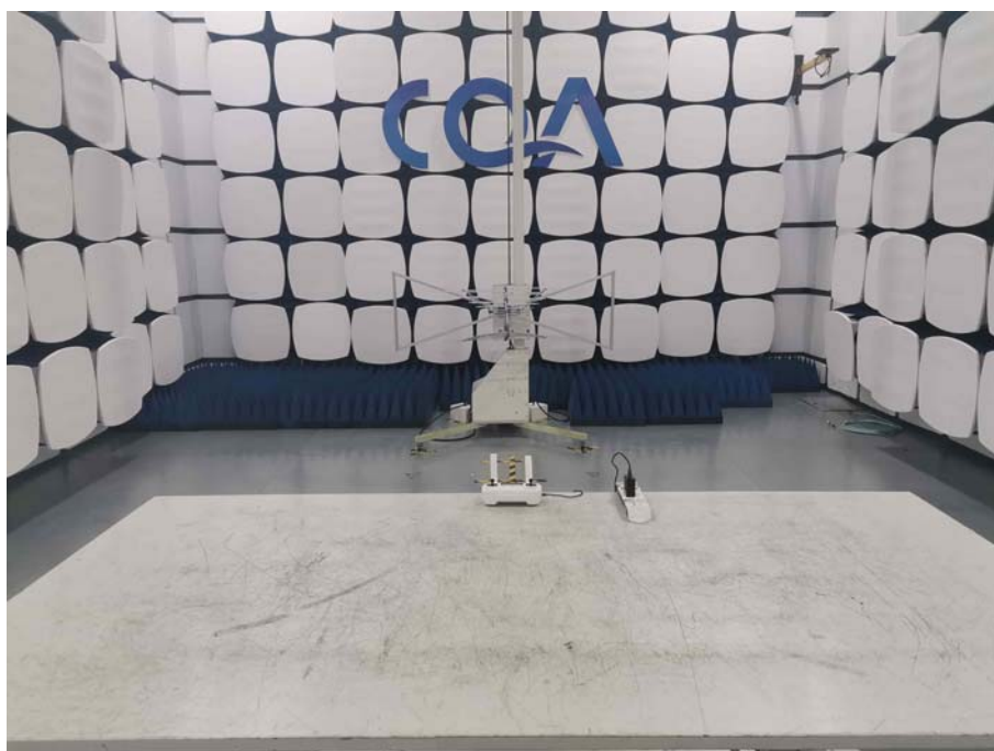
Radiated spurious emission Test Setup-2(30MHz-1GHz)
