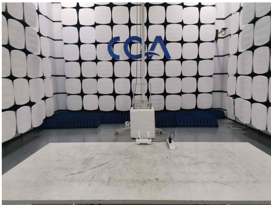
Radiated spurious emission Test Setup-1(Below 30MHz)
