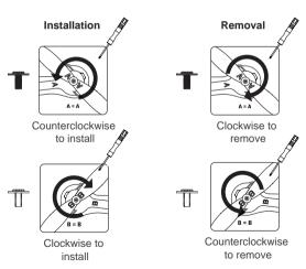
Note: Mind the differing colors of the A and B propeller screws!
