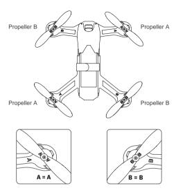
Installation: Before installing propellers for the first time, please check that each Propeller A is matched with motor A and each Propeller B is matched with motor B. Align the "I" with the flat side of the "D" shaped motor shaft. Then use the provided screws and screwdriver to secure each propeller. Propeller A's are paired with black propeller screws and are tightened counterclockwise. Propeller B's are paired with silver propeller screws and are tightened clockwise. (as shown below)
