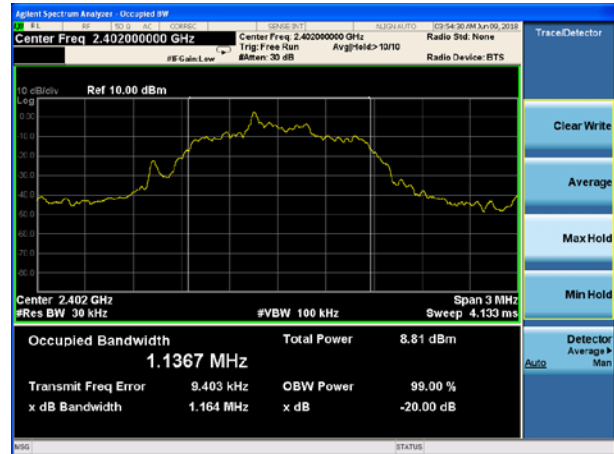
20dB Bandwidth plot on channel 39 (2Mbps)
