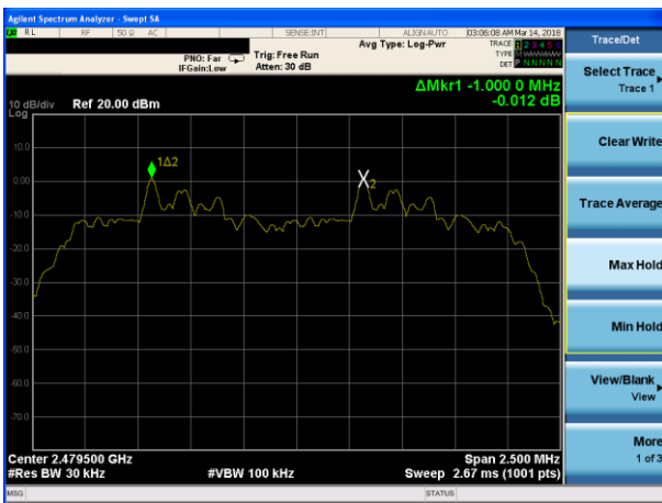
(3Mbps) Channel Separation plot on channel 77-78
