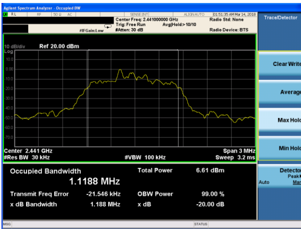
20dB Bandwidth plot on channel 39 (3Mbps)
