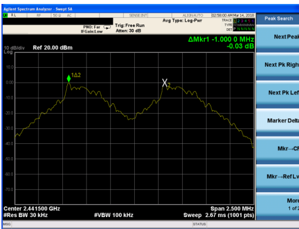
(1Mbps) Channel Separation plot on channel 39-40
