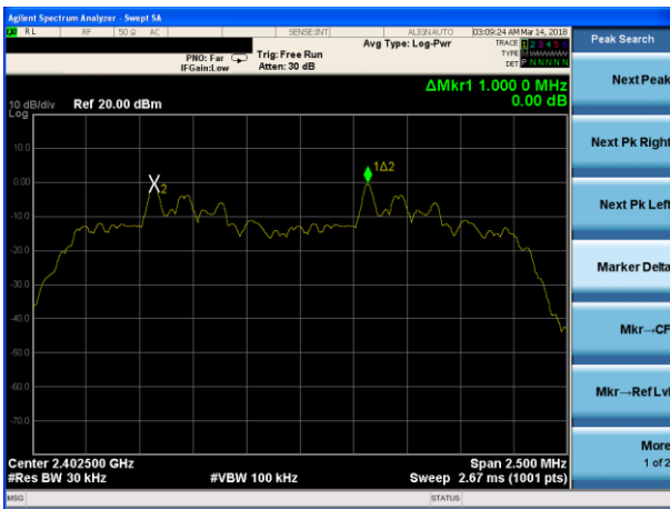
(3Mbps) Channel Separation plot on channel 39-40
